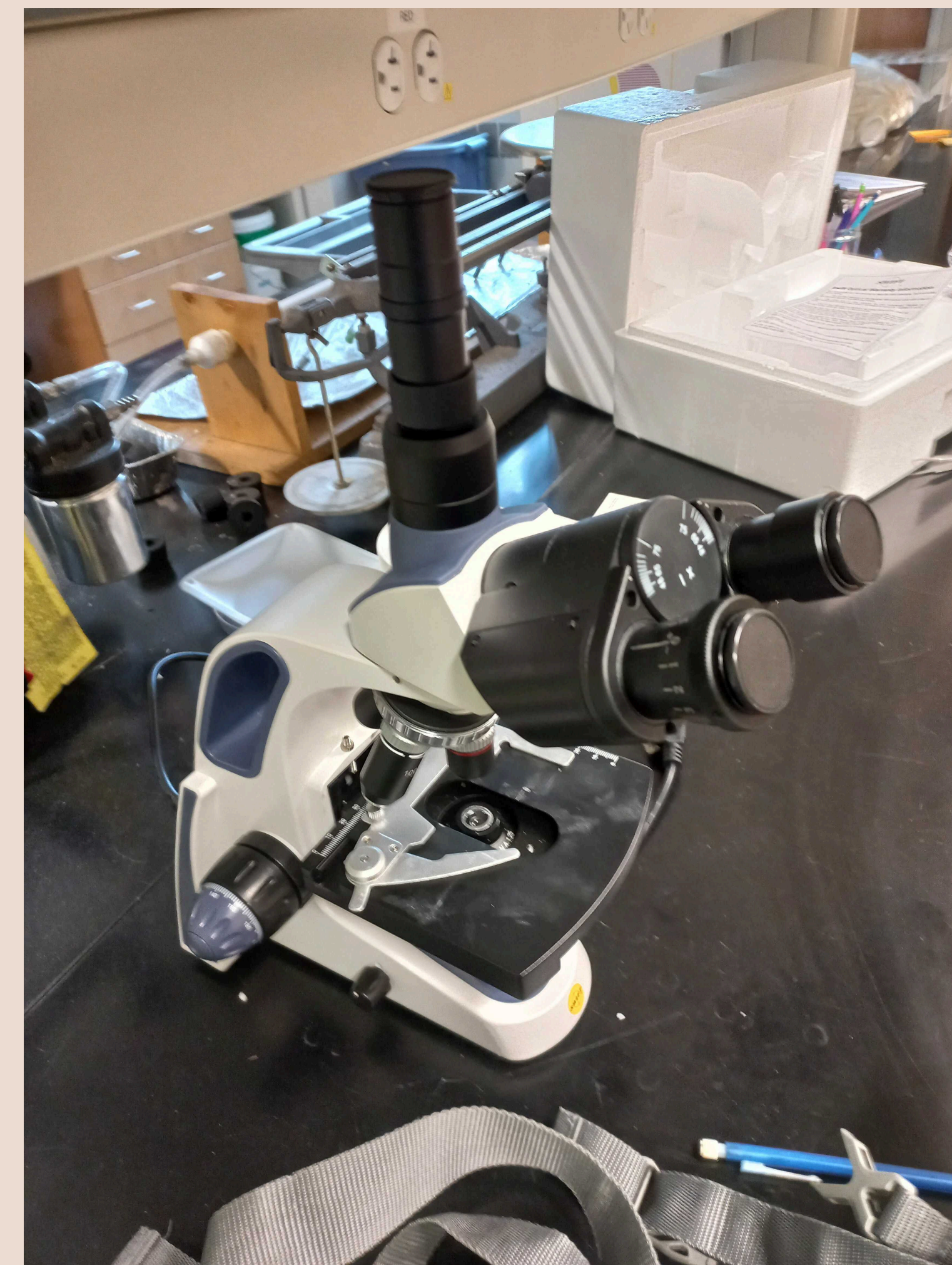
Figure 2. Swift 380T microscope used for microplastic identification
