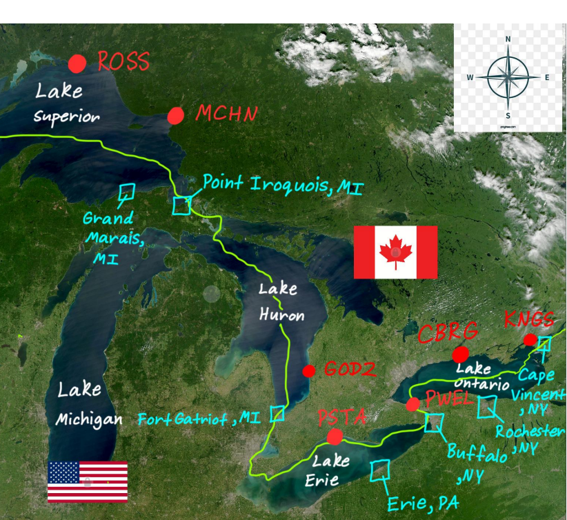
Figure 1: Map of GNSS-IR antenna stations (represented by red dots) and water height stations (represented by light blue squares) around coastal Great Lakes area.
