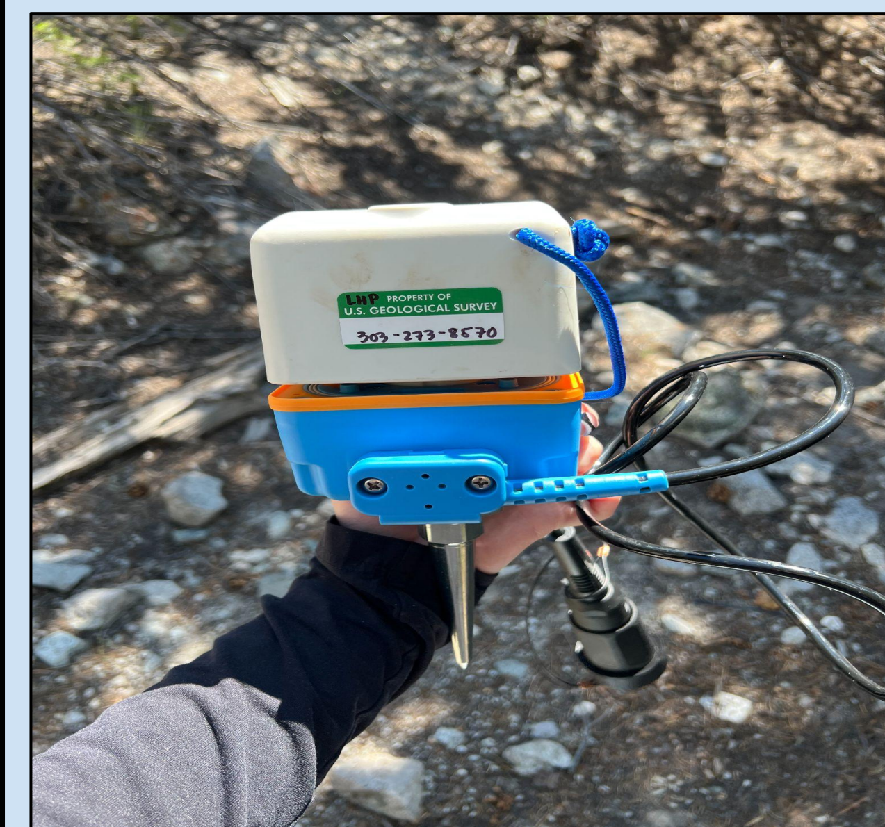
Figure 2. Seismic node about to be installed at the LSCCL site, Chalk Cliffs. Photo Credit: Natalie Aguilera
