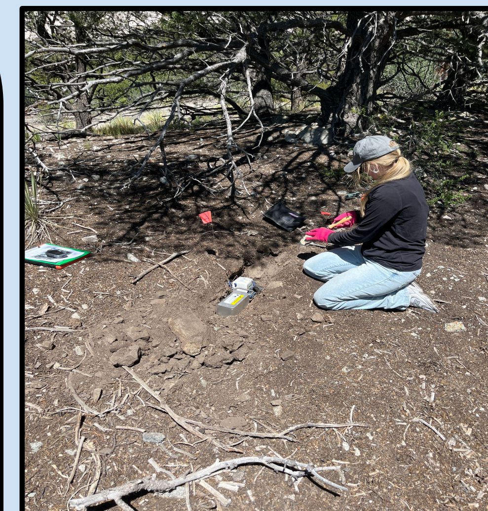
Figure 1. Site installation at Chalk Cliffs field site, June 2025. Seismic node deployed to capture subsurface signals associated with debris flow events. Photo Credit: Elaine Collins
